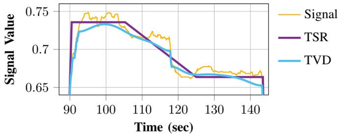
Fig. 2. Illustration of the curvature produced by TVD when approximating nearly constant regions of a signal. The proposed TSR algorithm approximates these regions with constant segments making the extraction of near-constant intervals easier.
