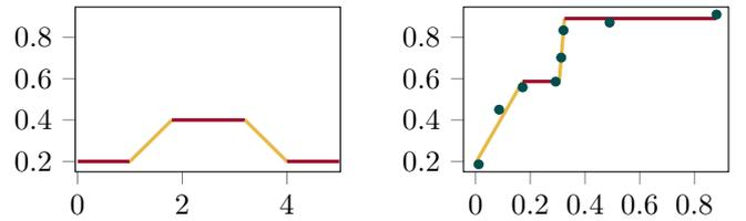
Fig. 3. Two trapezoidal signal examples. The left shows a prototypical trapezoidal signal shape. The right contains the optimum four-segment trapezoidal signal fit to the sample points. We use a broader definition of a trapezoidal signal: continuous alternating sloped and constant line segments. Each line type is colored differently for clarity.
