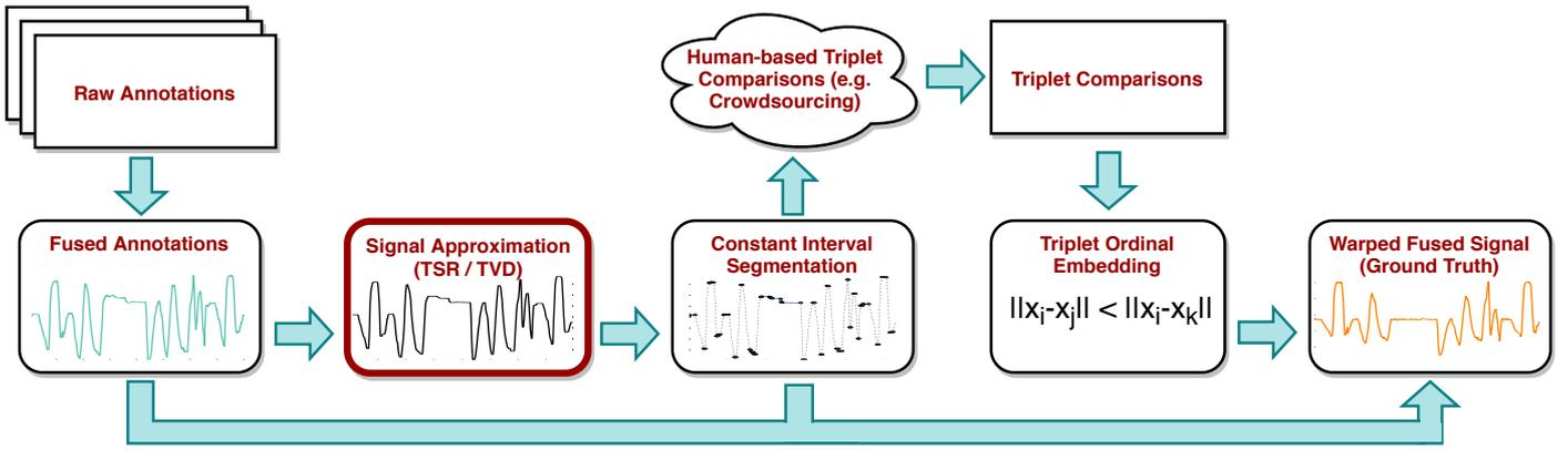
Fig. 1. Overview of signal warping algorithm first proposed in [1]. In this work, we explore using trapezoidal segmented regression in the signal approximation stage (highlighted) instead of total variation denoising.
